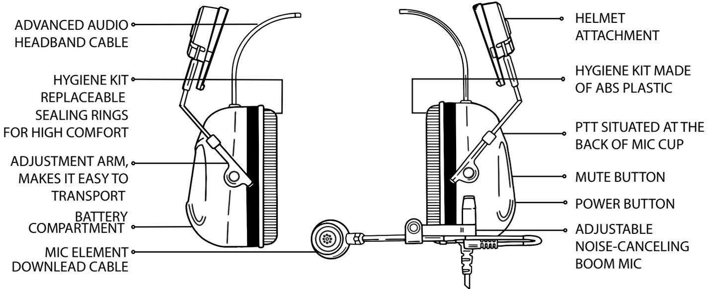
The SWATCOM 2Talk ARBORCOM Helmet Attached (AK6591) headset allows hands-free, full duplex encrypted communication between two matching headsets up to 200 meters apart
