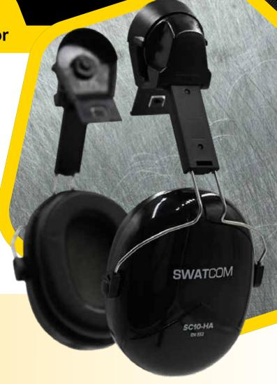
Market Segment Housing Material Weight Hearing Protector Attenuation Industry ABS (text) 234 g SNR 30dB, H 34dB, M 28dB, L 20dB<br/>SLC80 26dB, Class 5<br/>br/>NRR 23 dB Product code
